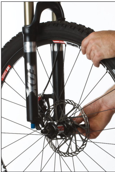
2. Slacken the front quick release and remove the front wheel from the fork.
