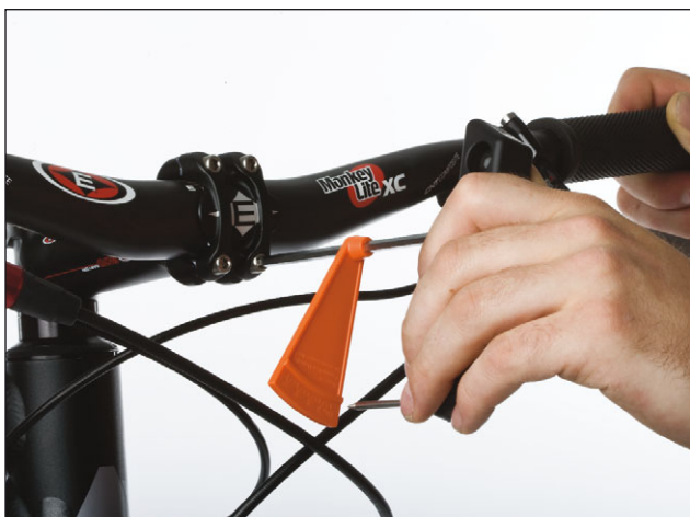
12. Now disassemble the handlebar. To do this slacken the bolts of the stem face plate with the Canyon Torque Wrench.
