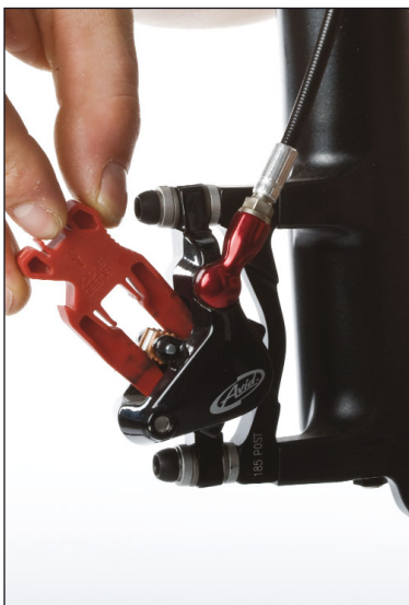
4. Push the plastic pad spacer between the brake pads.
