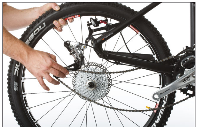
5. Now remove the rear wheel. In order to do this you'll need to slacken the quick release.
