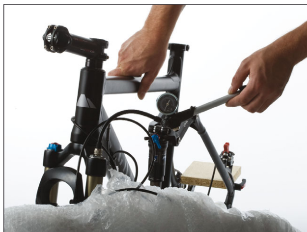
15. Deflate the fork with the shock pump and compress the fork so that the bike will fit into the BikeGuard in terms of height.
