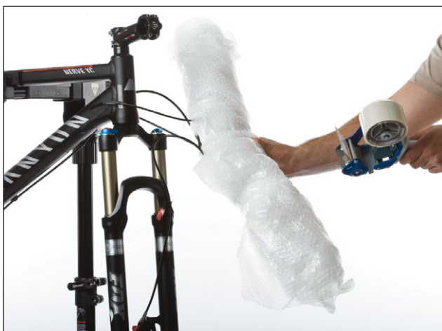
14. The handlebar should now be hanging down loosely by the shift cables and brake lines. Now wrap the handlebar in bubble wrap and secure it with adhesive tape.
